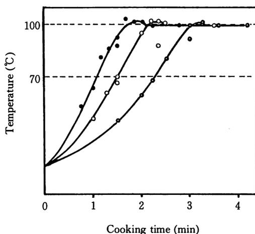
Fig. 1. Changes in the internal temperature of potatoes during microwave cooking as a function of part potatoes.
