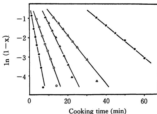
Fig. 3. Softening curves of microwave cooked potatoes at various temperatures.
