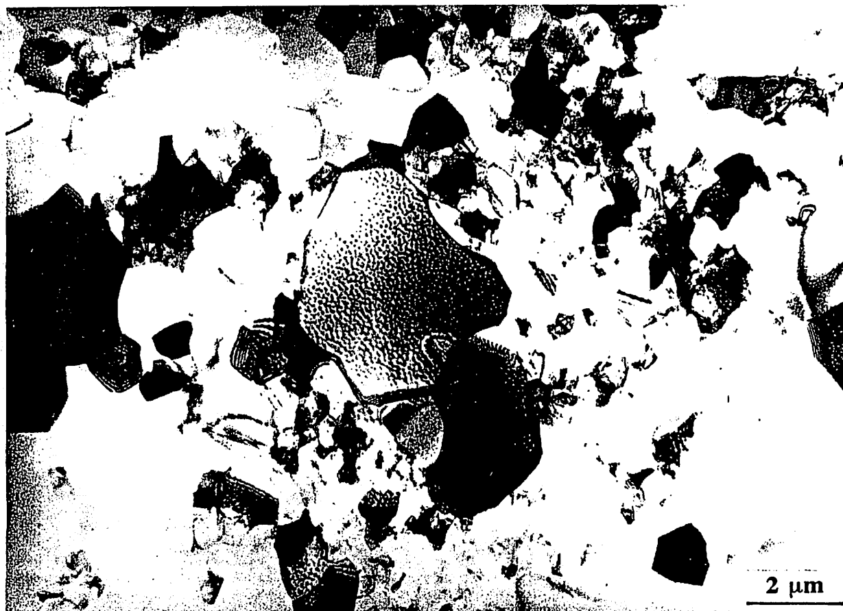
FIG. 5. Microstructure after annealing for 1 h at 533K.
