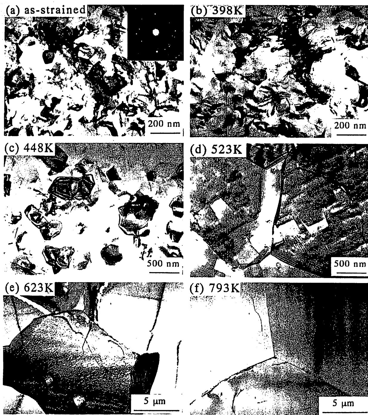
FIG. 1. Microstructures (a) in as-strained condition and after annealing at (b) 398K, (c) 448K, (d) 523K, (e) 623K, and (f) 793K for 1 h.
