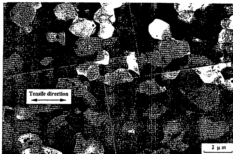
Figure 7 - Appearance of grains near the fracture tip of a specimen pulled to failure at 1970% at 473 K with an initial strain rate of 3.3 \times 10^{-2} \text{ s}^{-1} .
